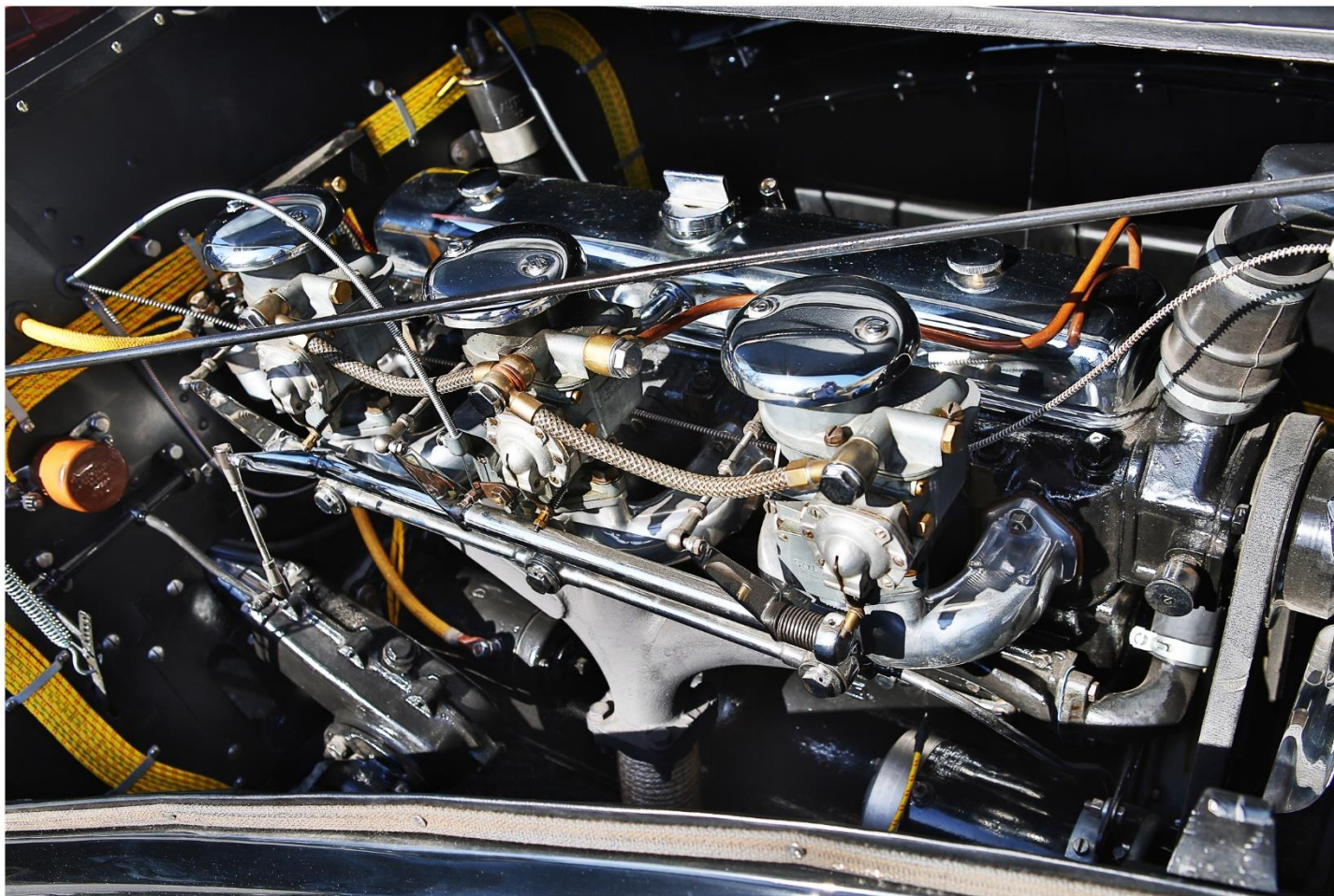
135M (Modife) Engine - 3.557cc - Triple Carburetors - 115bhp
